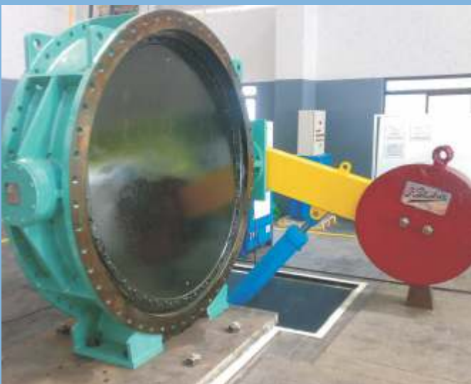
2100 mm Butterfly Valve for 2 X 2.45 MW Darna Power Project, Nasik, India
