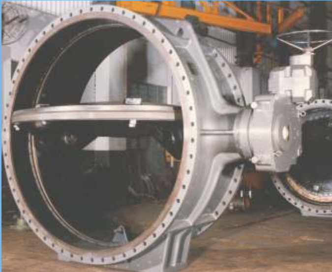
2400 mm manually operated Butterfly Valve, Brihan Mumbai Municipal Corporation, Mumbai, India
